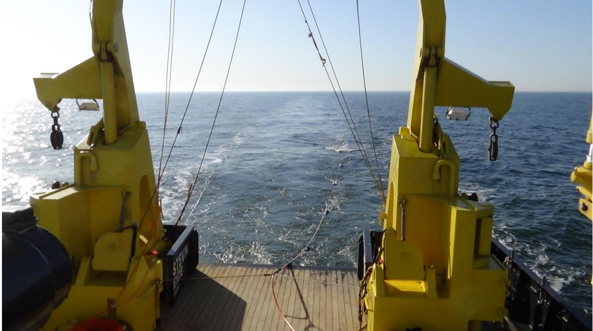
Figure 3 – GSO sparker and SC streamer towed behind the RV Simon Stevin
